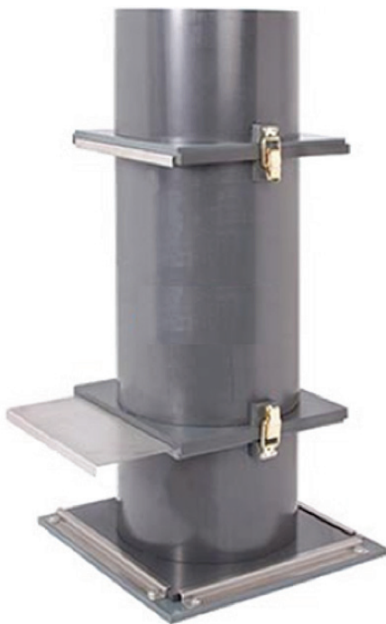
FIGURE A.5 ARRANGEMENT FOR STATIC SEGREGATION TEST IN ACCORDANCE WITH ASTM C1610
