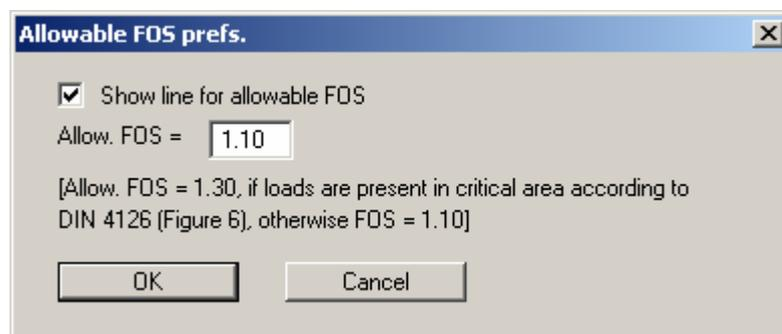
Just activate the line representation check box and enter the desired safety factor.
