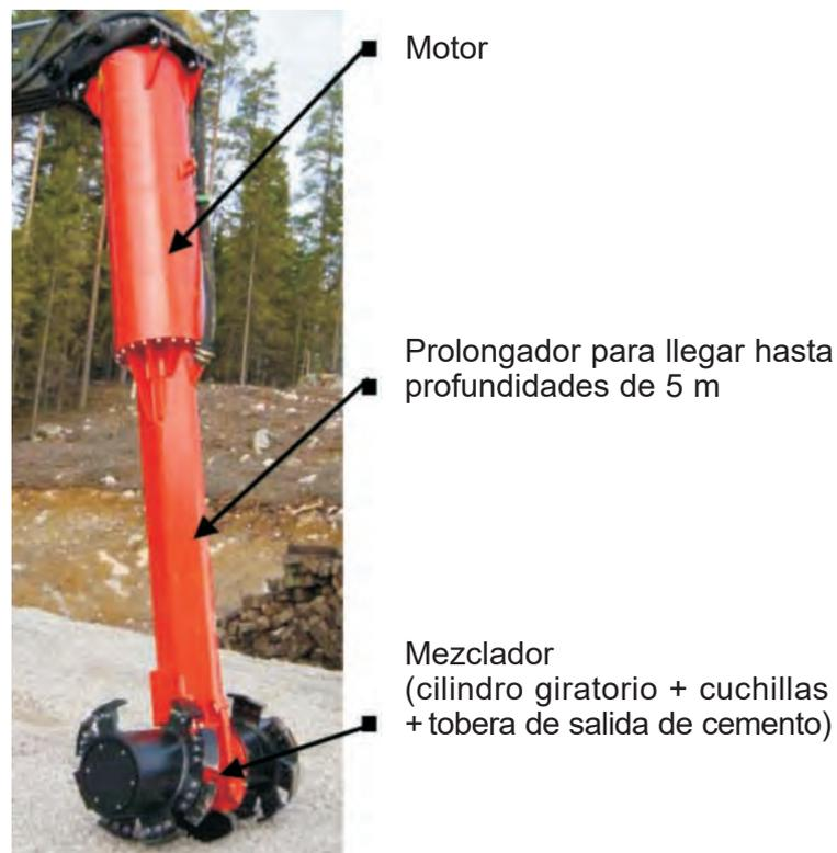
Figura 4. DETALLE DEL MEZCLADOR.
