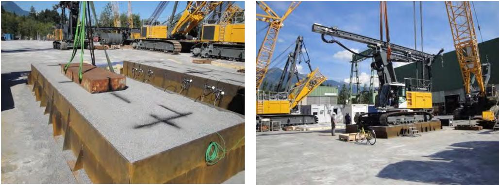
Fig. 13: Calibration of the soil pressure sensor (left) and positioning of the LRB 16 (right)
