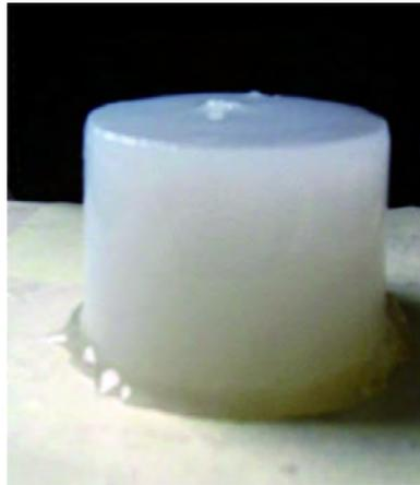
Sodium silicate gel modified with plasticity.
