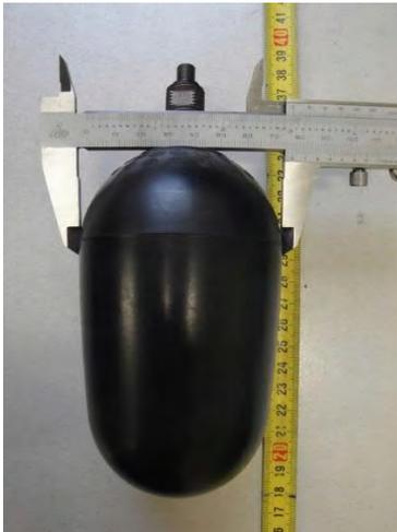
Fig. 9: Hydraulic accumulator bladder
