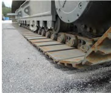
Fig. 21: Development of open gap under the crawler chain
