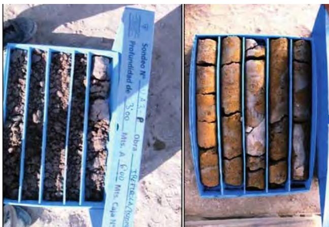
**Figura 41. SONDEOS BIEN Y MAL REALIZADOS DE LA MISMA COLUMNA.**
