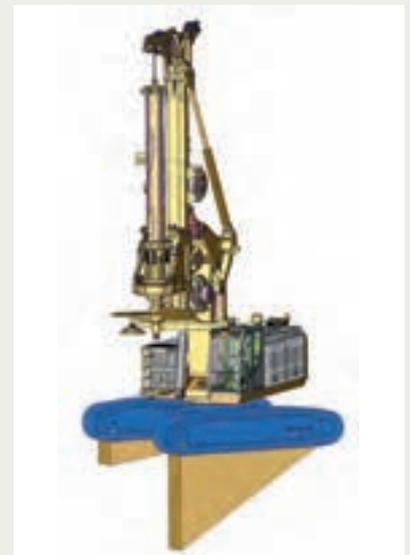
Principle representation of the surface pressure under the chains of a rotary drilling rig with Kelly equipment for different load positions
